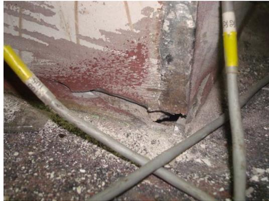
Figure 9. Fracture of West Column (North West Corner) at 2.7% Drift
